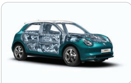
Iron Bone - Ultra-high Strength Steel Body Frame
